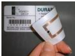
Figure 18.4: Passive RFID tag on back of a drug label (Courtesy CPTTM)
